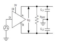
Figure 3. Driver Timing Test Circuit
