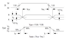
Figure 5. Driver Propagation Delays
