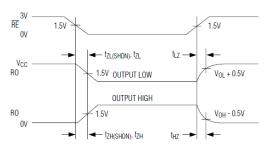
Figure 8. Receiver Enable and Disable Times
