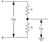
Figure 1. Driver DC Test Load
