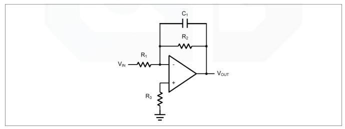
Figure 5. Low Pass Active Filter
