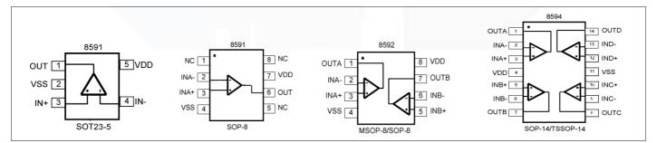
Figure 1. Pin Assignment Diagram
