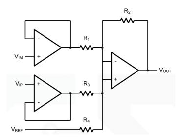
Figure 6. Instrument Amplifier
